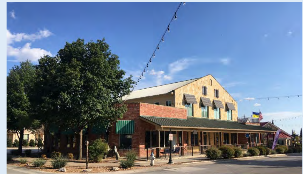
New commercial building in Gruene, Texas, with pedestrian-oriented building and site design – minimal or no front setback, storefront windows, wide sidewalks, building canopy, trees and landscaping, and covered outdoor seating. Parking is located at the rear and on the side away from the corner
